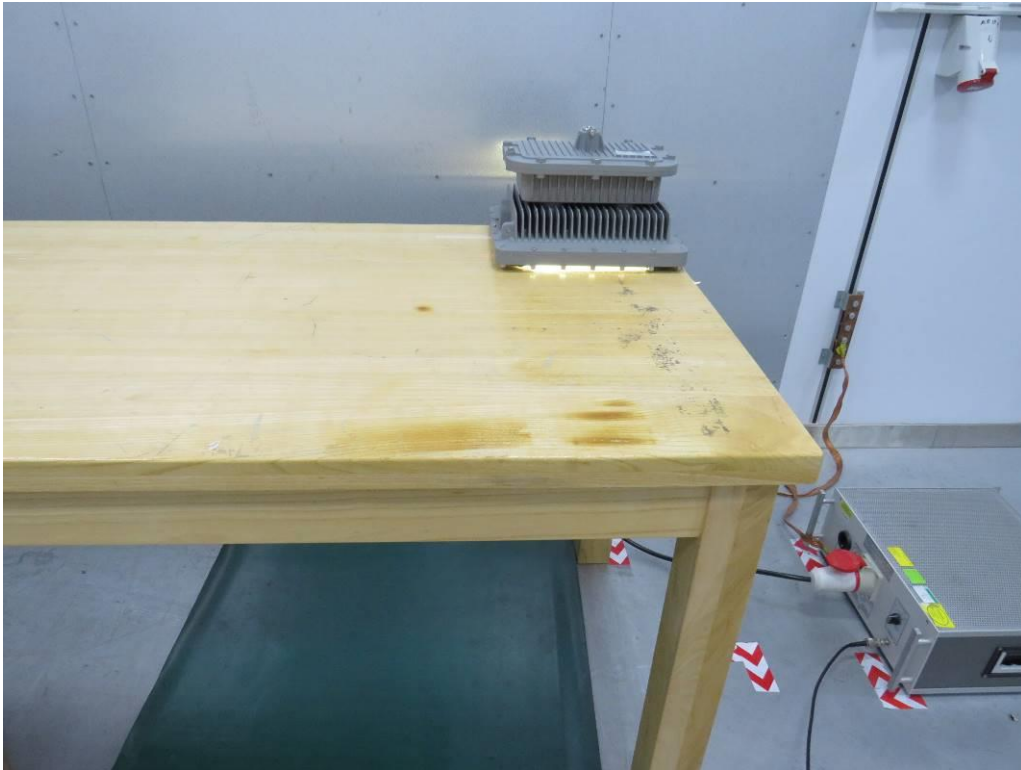
Conducted Emissions test setup photo
